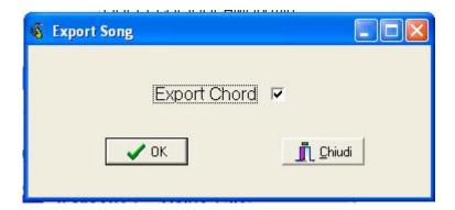
Selecting the option EXPORT CHORD, the related chords for each row will be displayed in the text file. Removing the checkmark for the option will export only the text as it is displayed on the screen.
